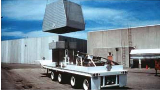
**Figure 3:** Package and trailer for road transport of used nuclear fuel: OPG (above); Areva (right).
